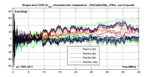
Typical impedance values becomes visible when we concentrate on few examples. The plots below show an in-quad and an out-of-quad example. The impedances are somewhat frequency depended, but if we concentrate on lower frequencies then the following circuit diagrams are indicative for these two examples.
