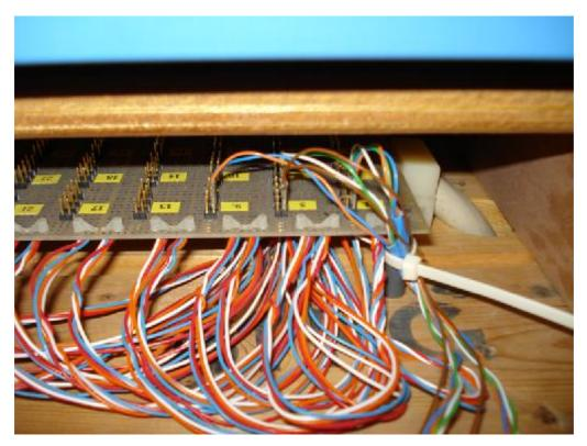
The quads are terminated at an bread board for interconnection with the measurement setup, and the wire pairs to be characterized were selected at random so that in-quad as well as out-of-quad combinations of wire pairs are in the selection.
