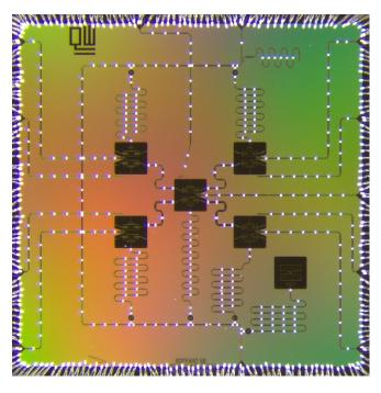
An optical image of a 6 qubit QPU device. Starting from the periphery, the wirebonds connecting the PCB to the QPU are visible. Most of the wirebonds are for grounding purpose, but the ones in correspondence to the on-chip CPW (black) lines are responsible to interconnect the various signals from the PCB to the QPU.
