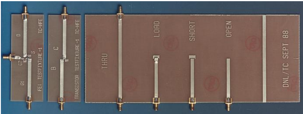
Fig 3.6 Calibration setup for two-port transfer measurements on transistors. The (SMD) transistor is mounted in the center of the fixture. The symmetry of the setup facilitates the positioning of reference planes in the center of the fixture using a Load, a Short and an Open
